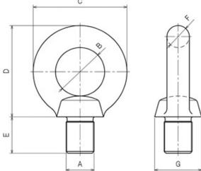
As a lifting KEY point, Eye bolt is the most common rigging equipment.
